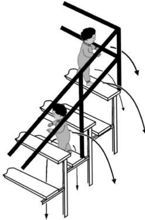
Figure 4: Inadequate guardrails and openings that permit falls from bleachers
